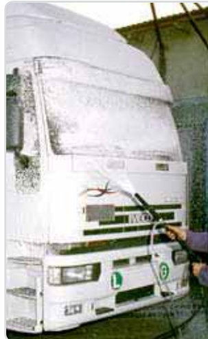
• Adjustable wax/detergent suction with double built-in tank (2 x 4,7 liters).
