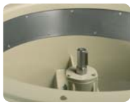
Aluminium strip to prevent sparks in accordance with standard EN-14986:2006
