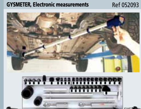
Light weight measuring arm with an easy to read digital display 400 > 2650 mm Measuring report Report Measured values Line 1 : 1890 µf Line 4 : 1890 µf Line 2 : 1670 µf Line 5 : 990 µf Line 3 : 1670 µf Car information Manufacturer: GYS Model: 2204 Year: 2014 License number: 2204 Serial number: 2204
